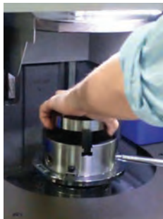
Step 1. Load tool into chuck
