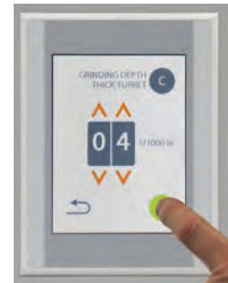
Step 5. Touch start to sharpen the tool
