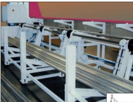
Bar loading magazines for the automatic loading of large-diameter round, rectangular and square material.
