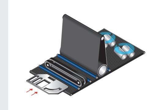
Dry grinding machine for mechanical removal of slag, deburring and edge rounding
