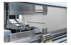
Quick-acting hydraulic clamping installed on the ram.
