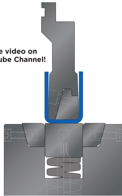
C2 – CHANNEL For deep channels when the channel bottom needs to remain flat.
